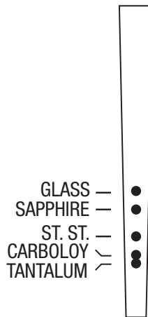
Figure 2 Effect of float position for the same rate of flow in Figure 1, but with increased pressure at the flowmeter outlet.
